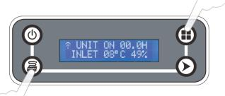
After the system beeps, the Wi-Fi icon will start flashing.
